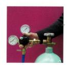
3. Attach regulator to new tank using wrench. Tighten firmly but do not over-tighten or you will damage the regulator.
